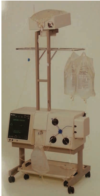
Figure 5 One of the earliest automated peritoneal dialysis machine introduced in the early 1990s.
