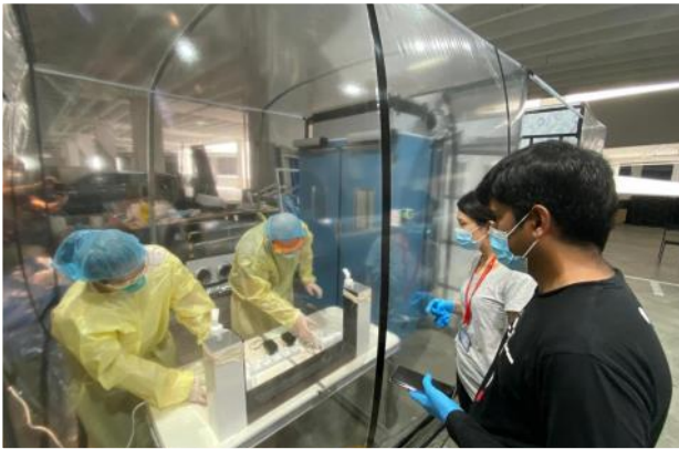
(From left) Dr Zibui Tan and Dr Hairil Rizal Bin Abdullah switching on the nebuliser to release the virus-containing droplets in the simulated patient room, while Dr Jye Yng Teo and Dr Balamurugan Periaswamy observe the release of the droplets from the nebuliser and time the duration of release
