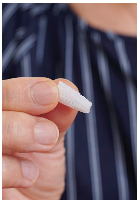
»»» The dental plug, which is 3D-printed and naturally biodegrades, includes a material that promotes bone growth.
