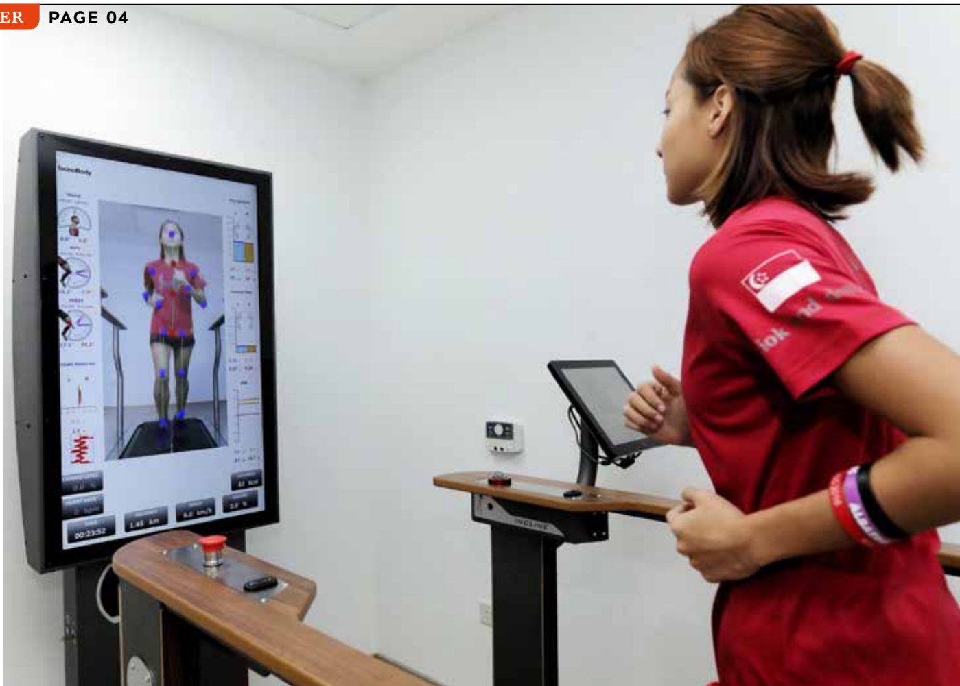
»» The Walker View treadmill uses virtual reality simulations and intelligent feedback to help patients improve their mobility, balance and fitness levels.
